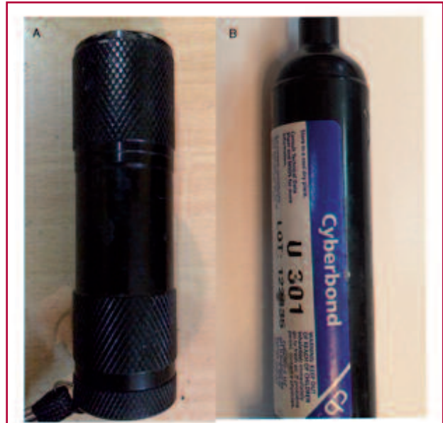
Fig. 1. A. Ultraviolet light source with a 1.5 cm diameter pen-shaped device (9 LED UV Mode blacklight flashlight). B. Cyan methacrylate tube.
